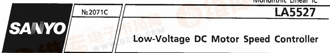
Especially suited for controlling speed of a low-voltage (3V min.) DC motor for cassette tape recorders, 8mm motion-picture cameras, record players
