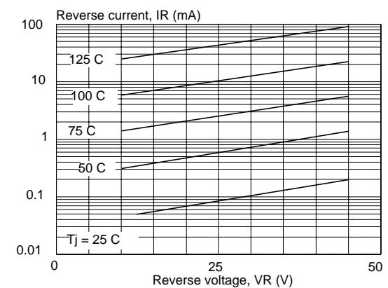
Fig.4. Typical reverse leakage current;  $I_R = f(V_R)$ ;
