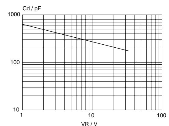
Fig.5. Typical junction capacitance;  $C_d = f(V_R)$ ;
