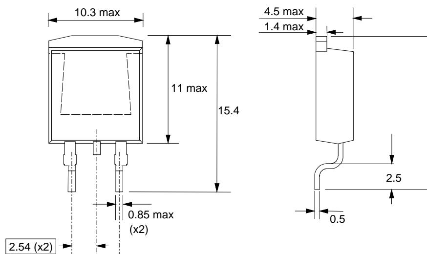
Fig.7. SOT404 : centre pin connected to mounting base.
