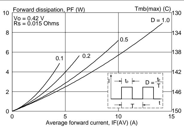
Fig.1. Maximum forward dissipation  $P_F = f(I_{F(AV)})$ ;
