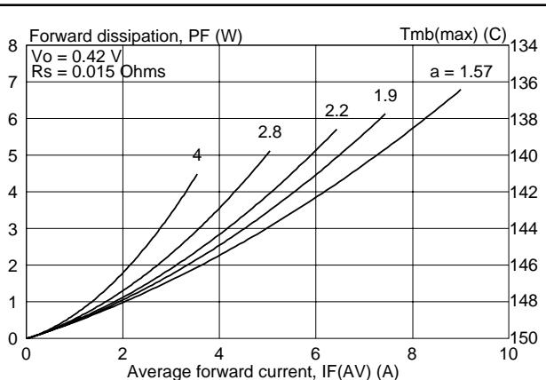
Fig.2. Maximum forward dissipation  $P_F = f(I_{F(AV)})$ ;
