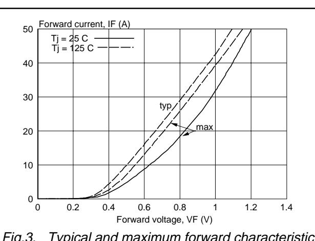
Fig.3. Typical and maximum forward characteristic
