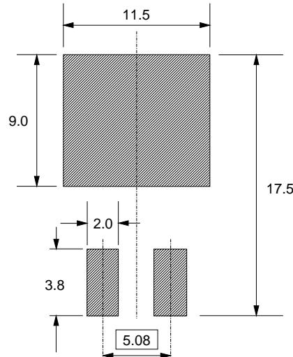
Fig.8. SOT404 : soldering pattern for surface mounting.
