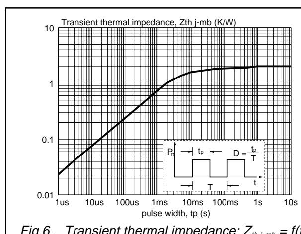
Fig.6. Transient thermal impedance;  $Z_{th,j-mb} = f(t_p)$ .
