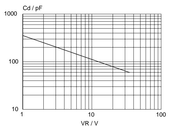
Fig.5. Typical junction capacitance per diode;  $C_d = f(V_R)$ ;  $f = 1 \text{ MHz}$ ;  $T_j = 25^\circ C$  to  $125^\circ C$ .
