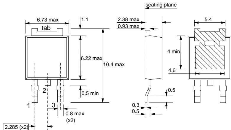
Fig.7. SOT428 : centre pin connected to mounting base.
