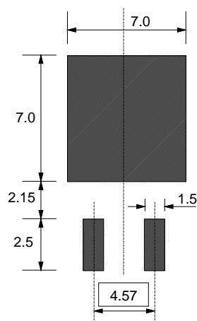
Fig.8. SOT428 : soldering pattern for surface mounting.
