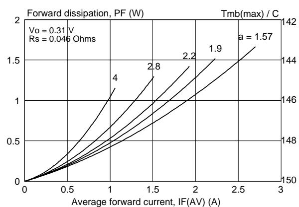
Fig.2. Maximum forward dissipation  $P_F = f(I_{F(AV)})$  per diode; sinusoidal current waveform where  $a = \text{form factor} = I_{F(RMS)} / I_{F(AV)}$ .
